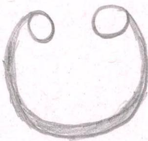
External circlips are used outside of the shaft or over the shaft. It is made up of a semi-flexible metal. They can be opened with the help of circlip pliers. These type of circlips prevent the lateral movement of the shaft and allows the rotating movement.
